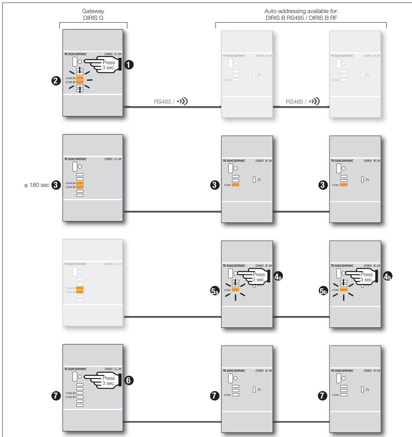
Note: During the auto-addressing process, the RS485 line is reserved for allocating addresses and no other exchange of data is possible at this time
