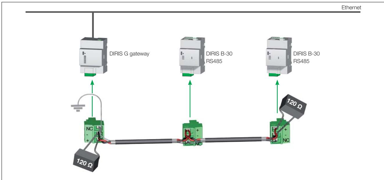
A LIYCY type connecting cable with a shielded twisted pair is required. In a disturbed environment or large network (in terms of length or number of products) the use of a type LIYCY-CY twisted pair with general shielding is recommended.
