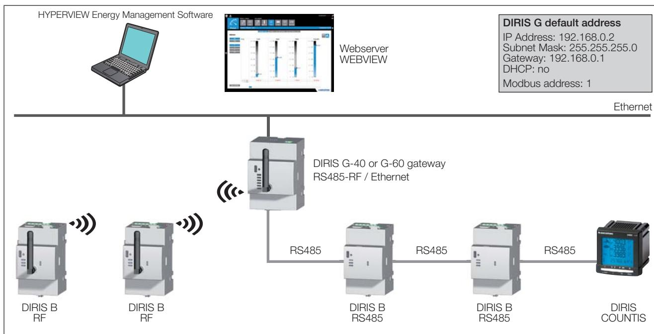
The DIRIS G-30, G-40, G-50 & G-60 gateways communicate via the Modbus protocol with the products connected to them. The DIRIS B which integrate radio communication are seen as Modbus slaves.
